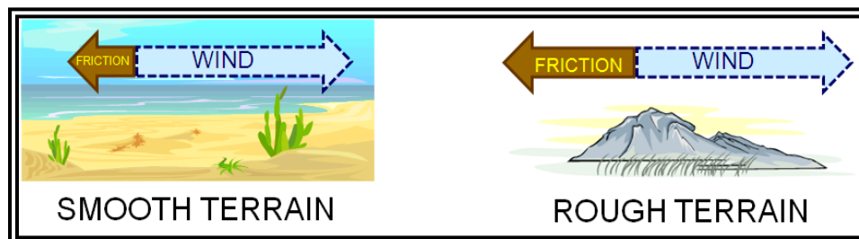
Figure 7-6. Friction Force Magnitude Variations with Terrain Roughness
