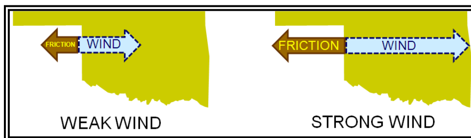
Figure 7-7. Friction Force Magnitude Variations with Wind Speed
